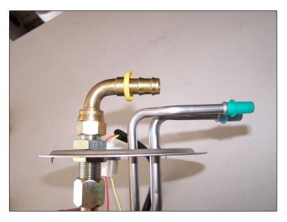
to work with them. It is helpful to put the end of the hose into a bucket of **HOT** water just prior to installing the fitting as this helps to soften the hose temporarily, making it easier to work with. We also recommend lubricating the barbed portion of the fitting to help the hose slide on more easily.
